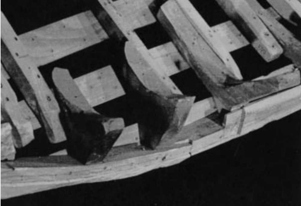
FIG. 7 – Detail of the model showing an oblique view of the scarf joint between the carved keel with integrated garboards (at right) and the heel of the stem (at left). Notice how the forward end of the carved keel yields to a standard garboard arrangement at the stem scarf (Photo: R. Chan, Parks Canada, RD-309X).
