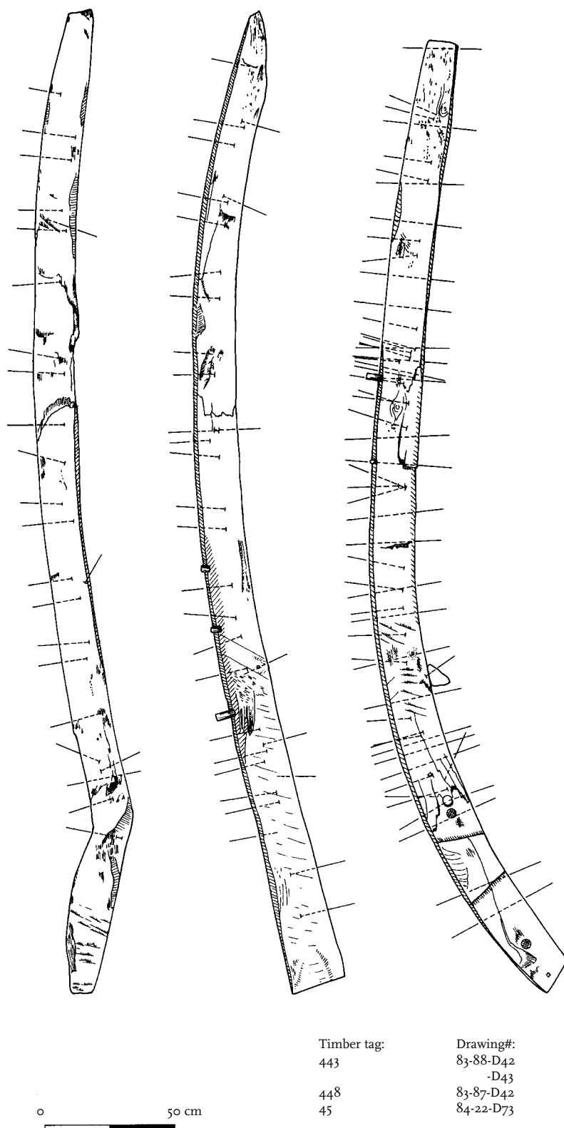
FIG. 28 – Drawings of three futtocks of different types illustrating the level of detailed archaeological recording of timbers conducted at Red Bay, including tool marks and fastener angles and depths of penetration (Drawings: J.C. Farley, C. Piper, R. Hellier, Parks Canada; 24M-95-103-9A).
