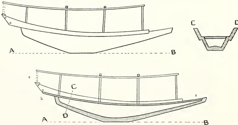
Fig. 199. — Profile and two sections.
