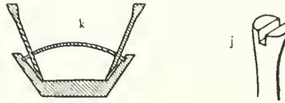
Fig. 192. — Rudder-posts.
