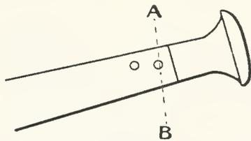
Fig. 58. — Slot joint on bow.
