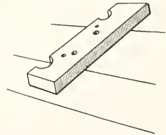
Fig. 65. — Rest for rudders.
