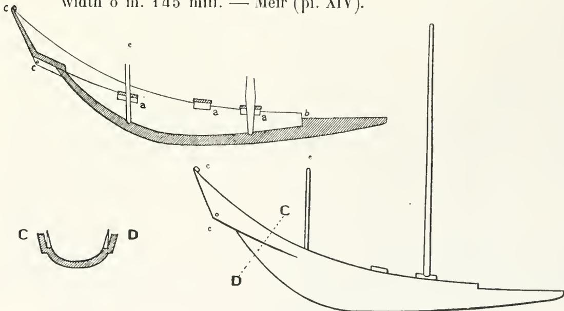
Fig. 204. — Profile and two sections.
