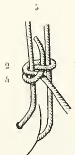
Fig. 210. — Rope-knot in hole, stern.
