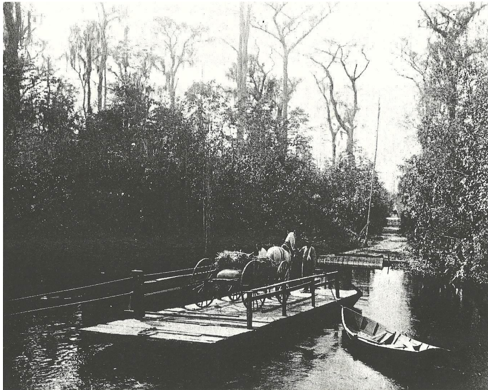
Ferry-flat used to cross the Oklawaha River in Florida, circa 1956. Power was provided this craft via an engine on the riverbank. John Perry, American Ferryboats (New York, Wilfred Funk, Inc., 1957), 7.
