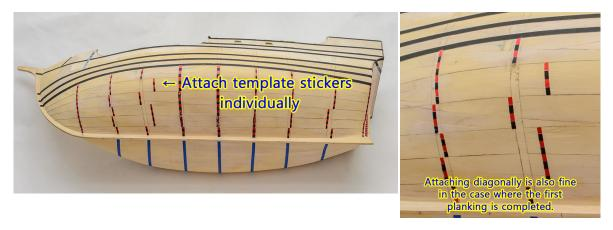
(4) Mark the width of each belt or plank. The usage is the same as the planking fan.
