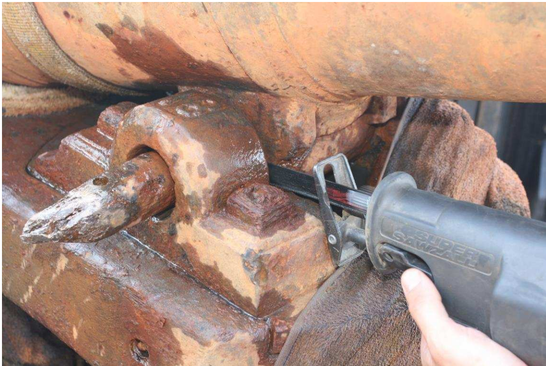
Figure 54. A reciprocating saw was used to cut through the lug bolt on ACC Oregon Carronade A. (Bajdek 2012)
