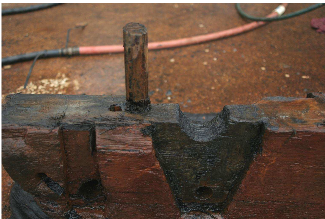
Figure 34. One half of carriage bed with exposed dowel. (Bajdek 2012)
