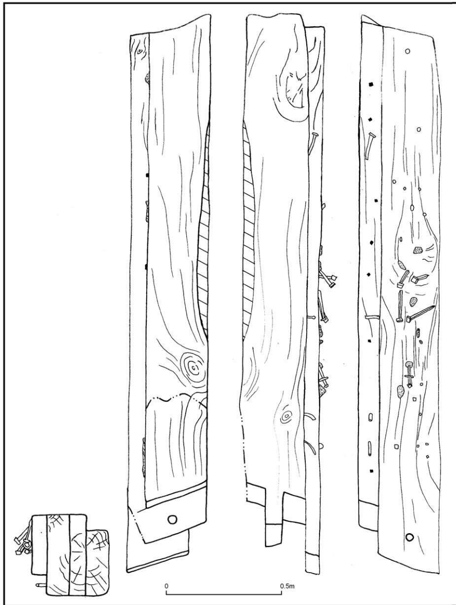
Figure 9. Timbers lifted from Str. [152], double rebated corner post [194]. (PCA Ltd)
