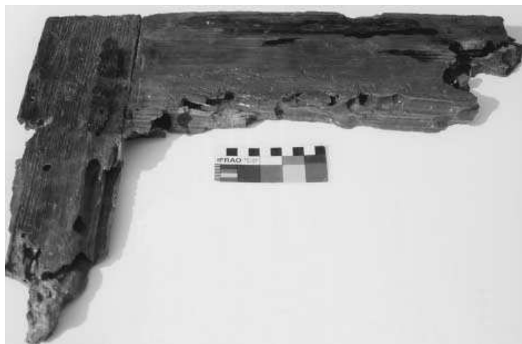
Figure 22. Window- or door-frame attacked by local wood-borer species. (M. Grosso)
