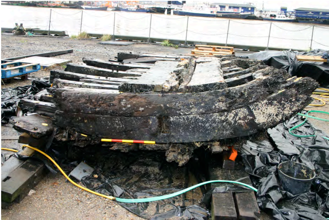
Figure 27 Furring requires more than just the removal of planks and adding additional frames and timbers (Photographed by Wessex Archaeology).
