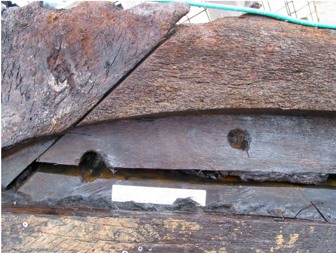
Figure 26: The stempost and rabbet of the Prince Channel Wreck . (Photographed by Wessex Archaeology)
